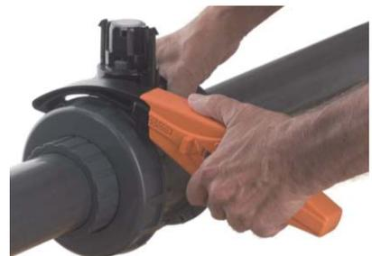
**6** Engage Wrench Key on Union Nut Groove to Tighten
